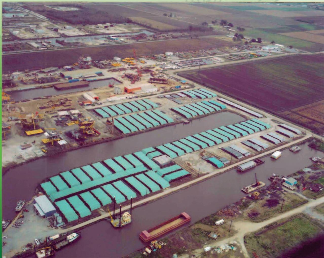
Pipe for the Cameron Hwy project is shown at the East Yard of The Bayou Companies at the Port of Iberia. This was one of the largest plant-applied pipe coating projects in the company's history with 150 miles of pipe. (Photograph courtesy of The Bayou Companies)
